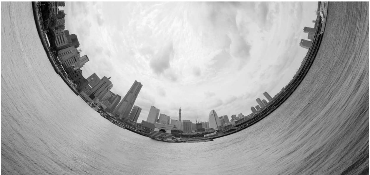
A wide-angle lens can distort the scale of images around the periphery of an image, and a fisheye lens exaggerates this distortion even more.
